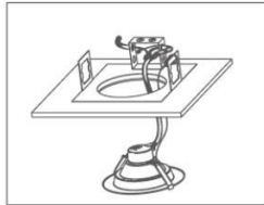
Bypass ballast & wire to j-box
